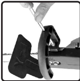
Parafuse a manopla com parafuso 8x16
